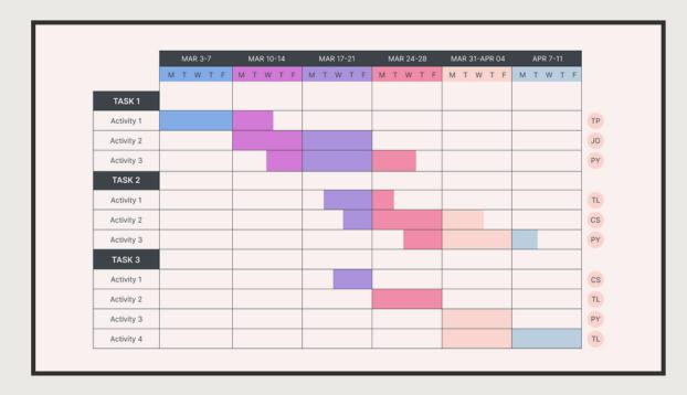
A Gantt chart is a project management tool that creates a visual timeline of a project's tasks, showing their start and end dates, duration, progress, and dependencies using horizontal bars on a bar chart
